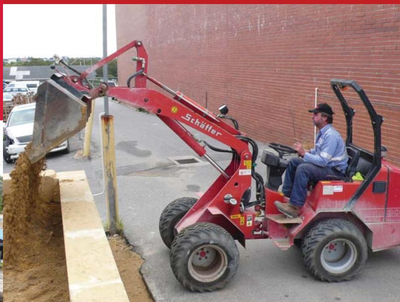
According to Robert, the Schaffer 3033 articulated loader is a pocket rocket, with plenty of brute strength despite its small size. "It's got a very good load capacity, it can lift around a tonne quite high.
