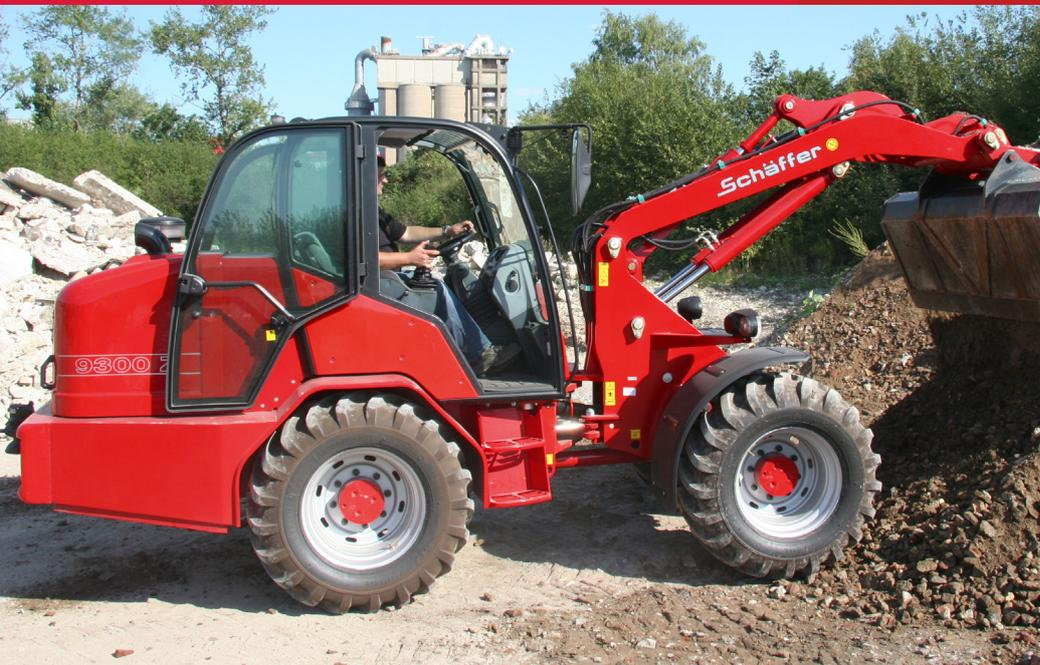
At 80kW (110hp), the 9300Z's Deutz water-cooled common rail intercooler turbo diesel engine was the most powerful but this did not equate to high diesel consumption. On the contrary, the 9300Z had the lowest fuel consumption – a feature that offers customers welcome savings in running costs.
